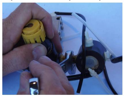
• Cut the ¼ black hose off the pilot valve. This is the air out to the clamp.
