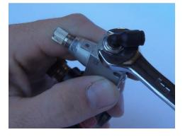
Install elbow fitting in regulator where connecting fitting was removed.
