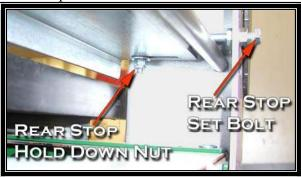
3. Remove the stop, but DO NOT adjust the Rear Stop bolts sticking out of the rear of the machine that butt up against the rear stop.
