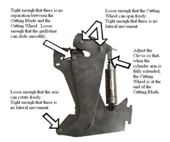
Cutting Wheel: This should be adjusted so the wheel can spin with little force. The wheel should have very little (if any) lateral movement. To adjust properly, tighten the machine screw then back off  $\frac{1}{4}$  turn. While securing the Phillips end of the machine screw, tighten the jam nut on the other side. Spin the Cutting Wheel. If the Cutting Wheel is too tight, loosen the jam nut, turn the machine screw  $\frac{1}{8}$  turn CW, and re-tighten the jam nut.
