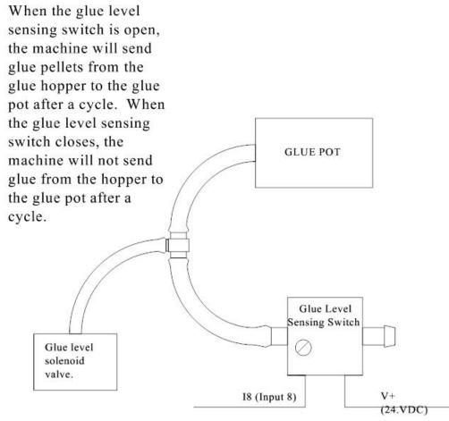
If glue level sensing switch adjustment screw is turned clockwise the switch will close with less air pressure so glue pellets are less likely to transfer when glue pot level is low.
