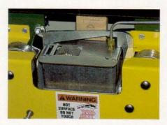
The transfer wheel is located in the top of the glue pot. It applies glue as the board is pushed through the machine. The glue level sense tube is a black poly tube that is pressed firmly into the fitting on the control box.
