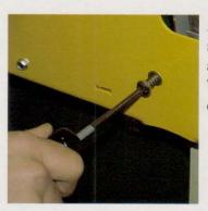
Adjust the width with the screw with a spring under the head. It should also be adjusted until the tape has a slight drag. The spring keeps the adjustment from changing with use.
