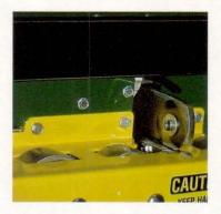
The guillotine will come forward and block the banding process during warm up periods and when the machine is asleep.
