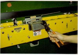
Reverse this procedure to install a glue pot, making sure it is installed all the way back onto the rear of the hot plate. Fill the empty glue pot with glue pellets to the top of the transfer wheel axle prior to installation.
