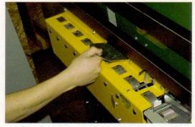
4) Control Box: Located on the right hand side of the machine. The portion visible in the front consists of three LED lights and two push buttons.
