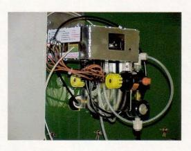
The regulator closest to the front of the machine sets how much air is sent through the pressure sense tube. The gauge next to it should be set at approximately 5 1/2 PSI. The regulator towards the rear should be at six full turns to the right from being completely off.
