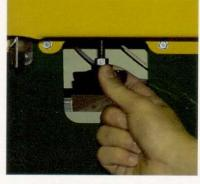
2) Release the glue level sense tube by pushing in the ring on the control box fitting while simultaneously gently pulling on the poly tube.
