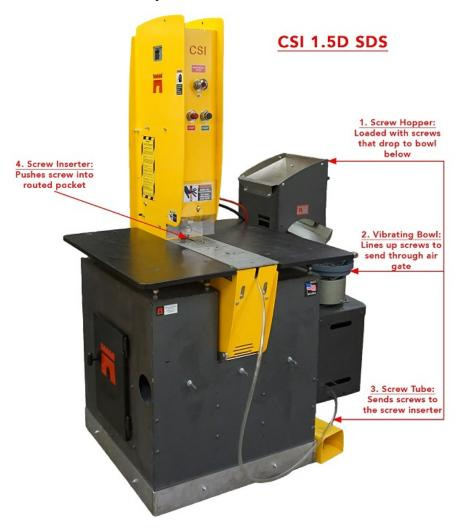
The CSI's new SDS is even simpler than the original, needing fewer adjustments, and is extremely low maintenance.
