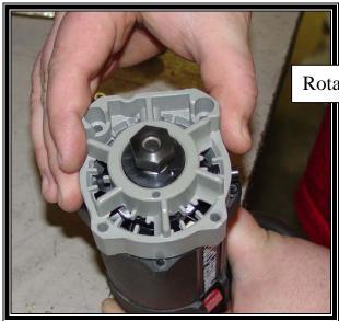
Rotate the motor front  $90^{\circ}$  counter-clockwise.
