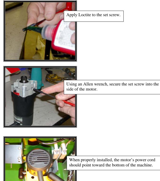
When properly installed, the motor's power cord should point toward the bottom of the machine.
