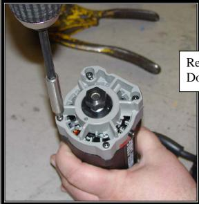
Remove the four screws from the front of the motor. Do not separate the motor front from the motor body.
