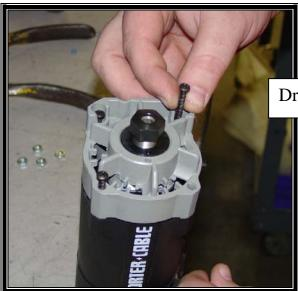
Drop the screws back into the motor front.
